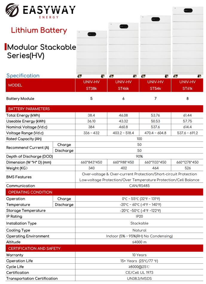
The recommended and max. continuous operation current is for a battery cell temperature within 10~40°C to consider, out of such temp. range will cause a derating on operation current.
