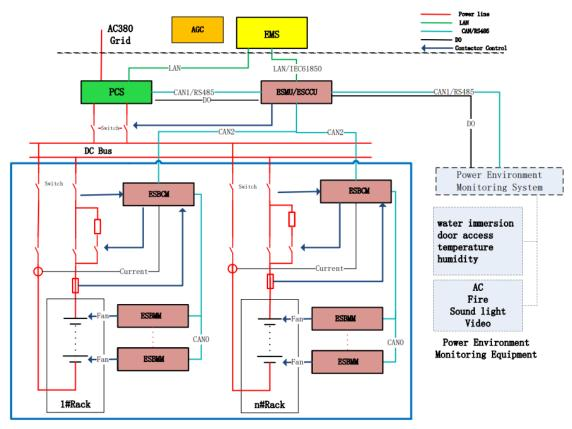
Figure 1 System Architecture of BMS
