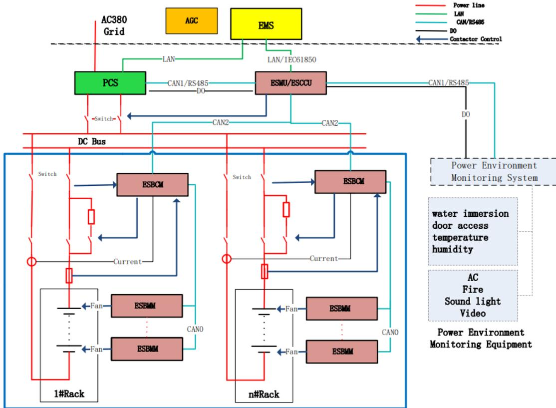
Figure 1 System Architecture of BMS
